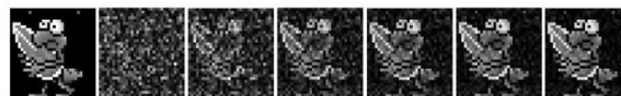
Figure 3: Watermark logo: Original and recovered from GA solution after low-pass filtering the watermarked image with \sigma = 50, 60, 70, 80, 90, 100 .
